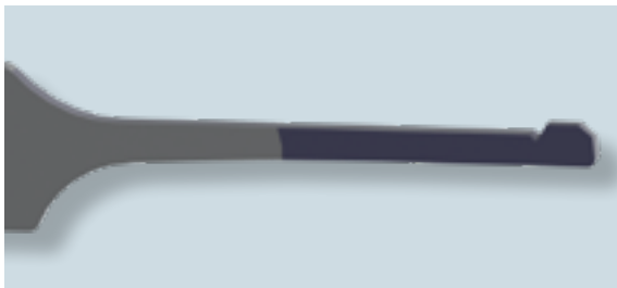
Fig. 2: The blade and the spring form a single unit. This solution allows simple handling despite the miniature dimensions.
